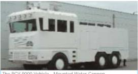
The RCV 9000 Vehicle - Mounted Water Cannon
