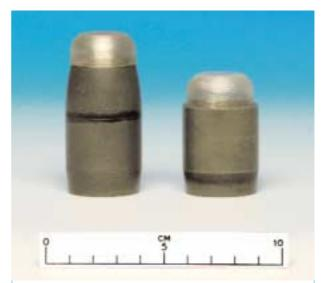
Medium calibre variants (of different mass and aerodynamic properties) of 37 mm DIP concepts, showing the carrier body and irritant payload in the nose, within a frangible cap. There has been no decision yet on the preferred calibre of the projective, but a smaller calibre option would be entirely frangible with no carrier body.
