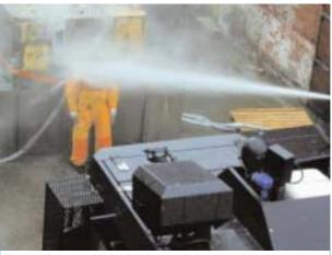
Figure 1: Restrained Hybrid III dummy during water impact
