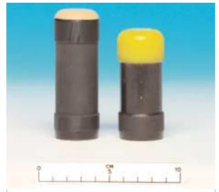
Development prototypes of the AEP, showing the incorporation of novel materials into the impact face of the projectile to provide frontal energy absorption. The projectile on the left incorporates voids in the nose; the projectile on the right employs energy attenuating materials alone.
